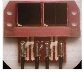
The solar cells are key to determine the performance, robustness and reliability of a sun sensor. All the sun sensors produced by Airbus are made from the same solar cells from OSI and benefiting from Airbus skills in the procurement and qualification of opto-electronic components for space application.
