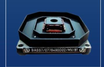
BASS7, BASS17, BASS17R and BASS17R GEO are simple analogue sensors: angle measurement is obtained by comparing intensities produced by two silicon solar cells mounted on opposite sides of a pyramid. The body of the equipment gives a +/-90° sensor fine field of view on each measurement axis. For specific programs, the coarse FOV (Field of view) can be reduced by adding specific external baffles to protect from straylight.
