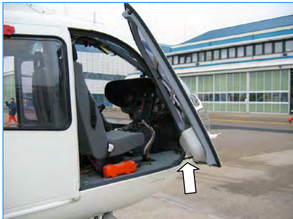
To enlarge the door opening, unhook the gas pressure spring.
