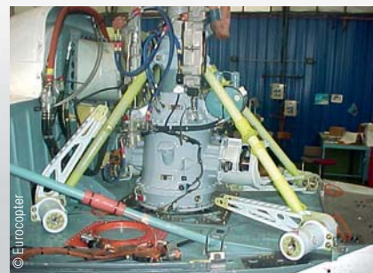
The "flapping masses" are installed on the attachment fittings of the MGB struts.
